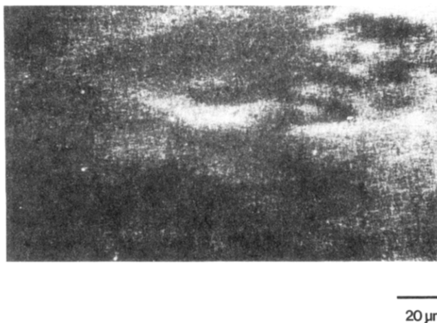
Figure 2. Optical micrograph of MBPE-9, taken through crossed polars at 70 °C immediately on cooling from the isotropic melt.
